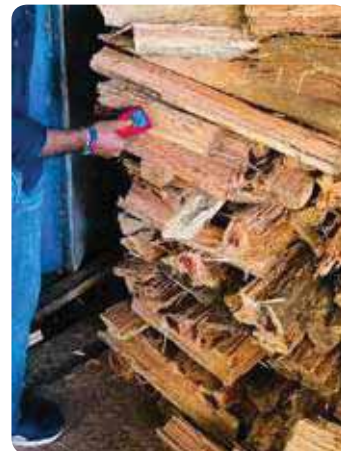
Fire-wood moisture determination
